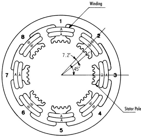
Fig. 6-1 Stator
