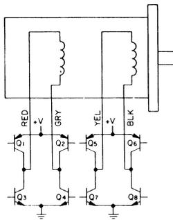
Fig. 8-3 Bipolar Method
