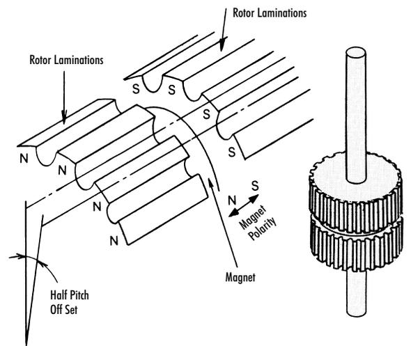
Fig. 5-2 Rotor Construction
