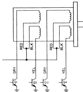
Fig. 8-4 Unipolar Method
