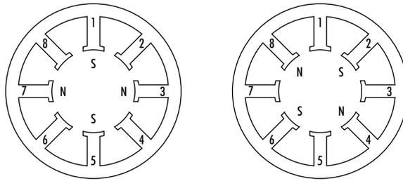
Fig. 6-2 Rotational Magnetic Field Generated by Phase Sequence
