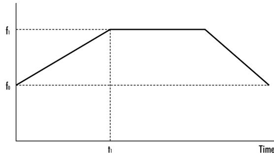
Fig. 9-4 Linear Acceleration
