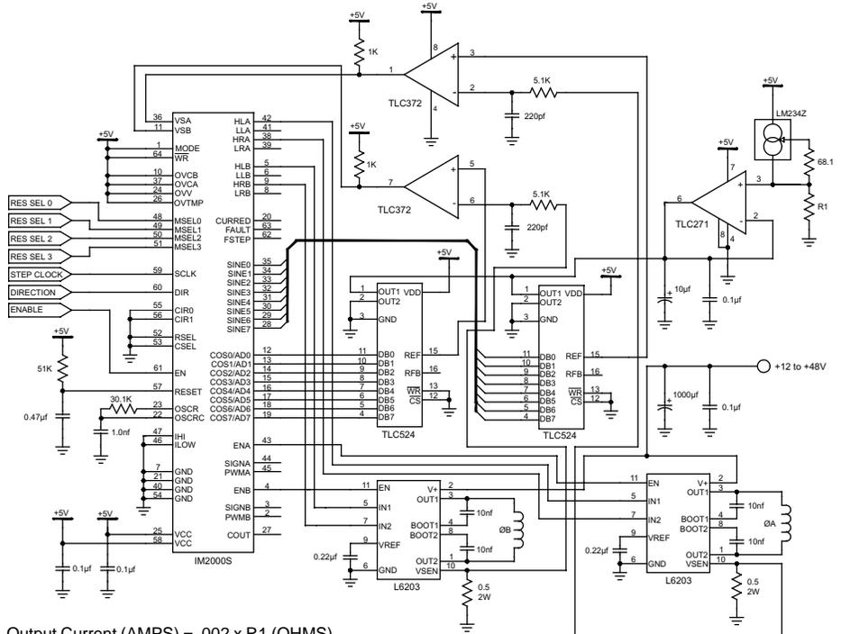
Output Current (AMPS) = .002 x R1 (OHMS)
