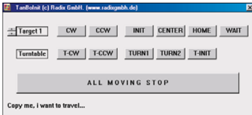
Figure 2. Initialisation program for calibrating the arms and turntable.
