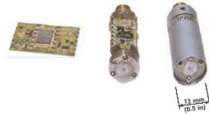
Figure 10 – signal filtering circuits from the TP200 strain gauge probe.
