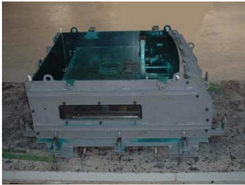
Mould is fixed on a vibrating table
