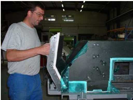
The part is removed from the mould 48 hours after casting
