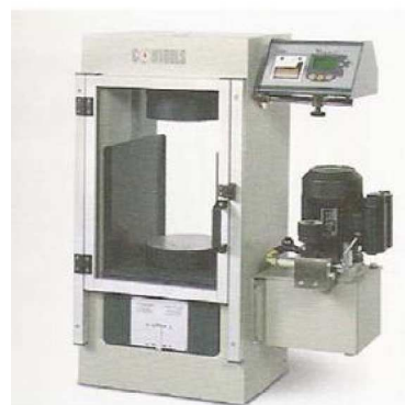
Machine for compressive and flexion tests 4 columns Max. load : 2 000 kN
