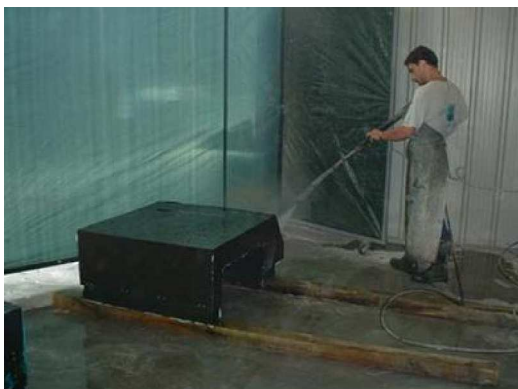
The high-pressure cleaner removes the demoulding agent
