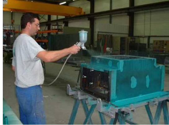
Spraying on demoulding agent
