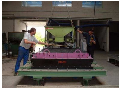
The hopper contents are poured into the mould
