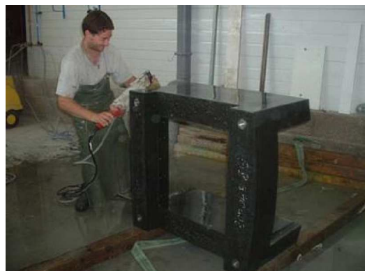
Corners are smoothed off with a flexible grinder
