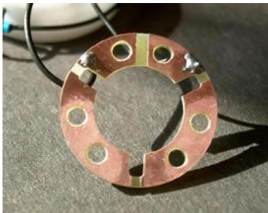
copper clad circuit board. The wholes were drilled and then small sections of copper were removed from the narrow portions of the board with a 1mm end mill before the shape was cut out with a PCB routing bit.
