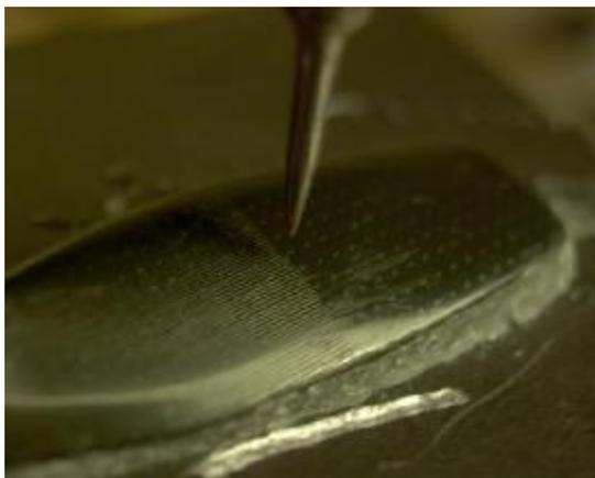
wanted. The picture to the left shows the digitizer in action. The small dots are where the digitizer has touched the surface. It has to overcome the force of the spring before triggering so there is some mild deformation.
