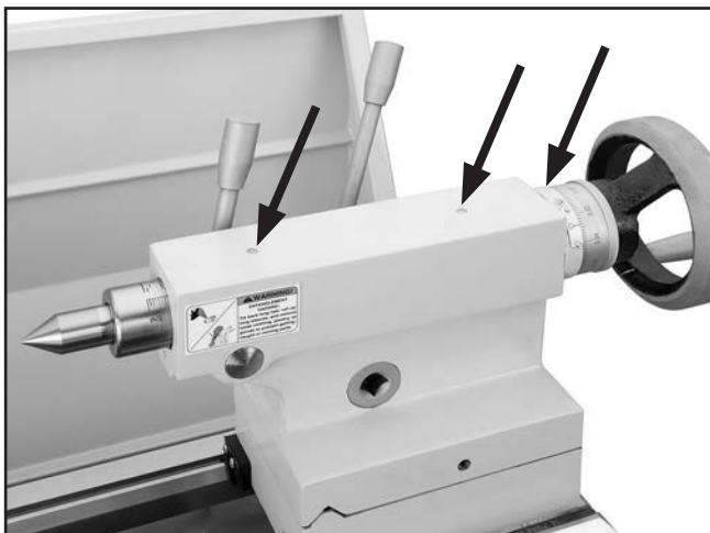
Figure 78. Tailstock ball oilers.
