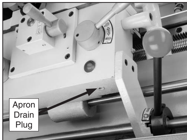
Figure 85. Apron drain plug.
