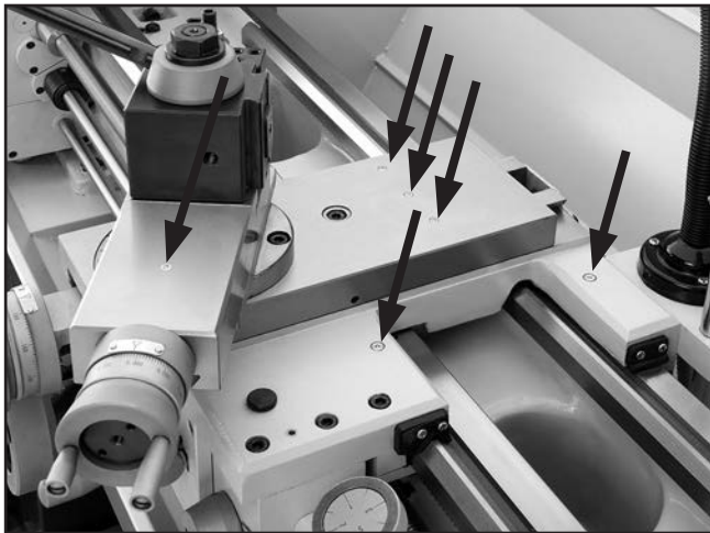
Figure 77. Saddle and slide ball oilers.
