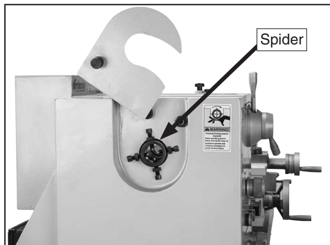
Figure 45. Spider assembly located on the outboard spindle.
