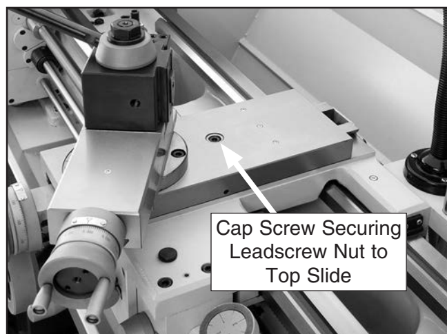
Figure 100. Location of cap screw that secures the leadscrew nut.
