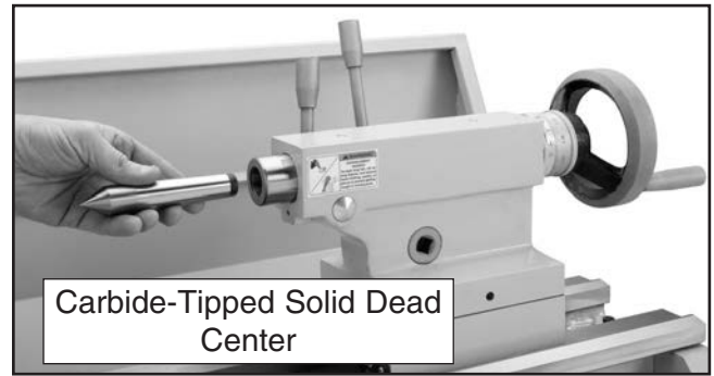
Figure 35. Inserting a carbide-tipped dead center in the tailstock.
