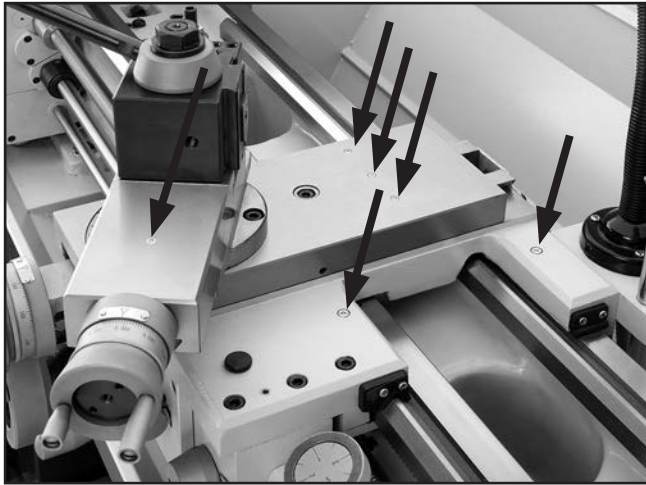
Figure 84. Saddle and slide ball oilers.
