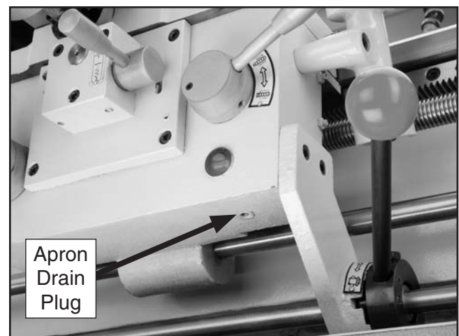
Figure 92. Apron drain plug.
