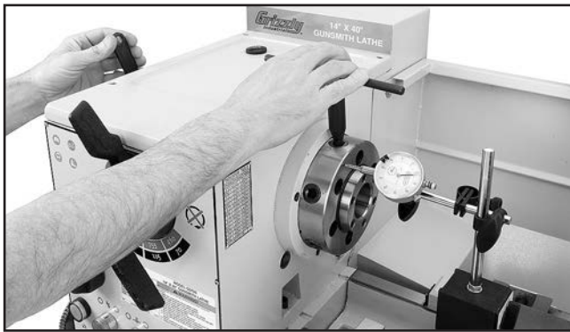
Figure 110. Adjusting spindle bearings.
