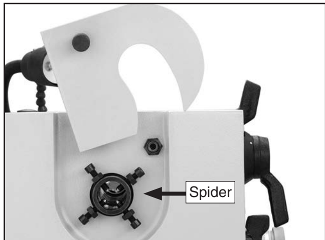
Figure 46. Spider assembly located on the outboard spindle.
