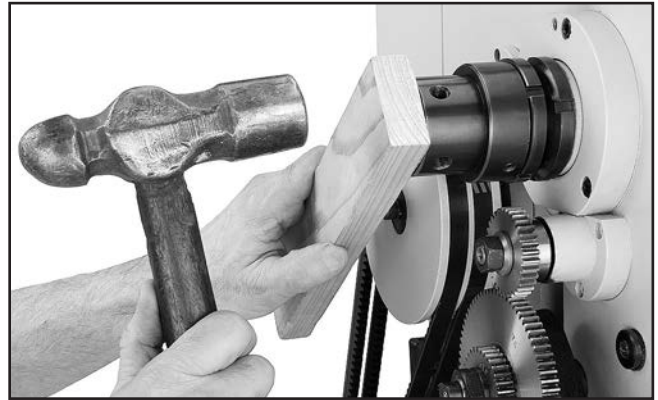
Figure 108. Un-seating spindle bearings to introduce spindle end-play.
