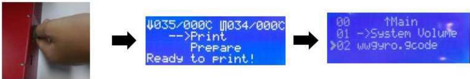
Insert SD card → push-turn key → Select from the memory card → Files to print
