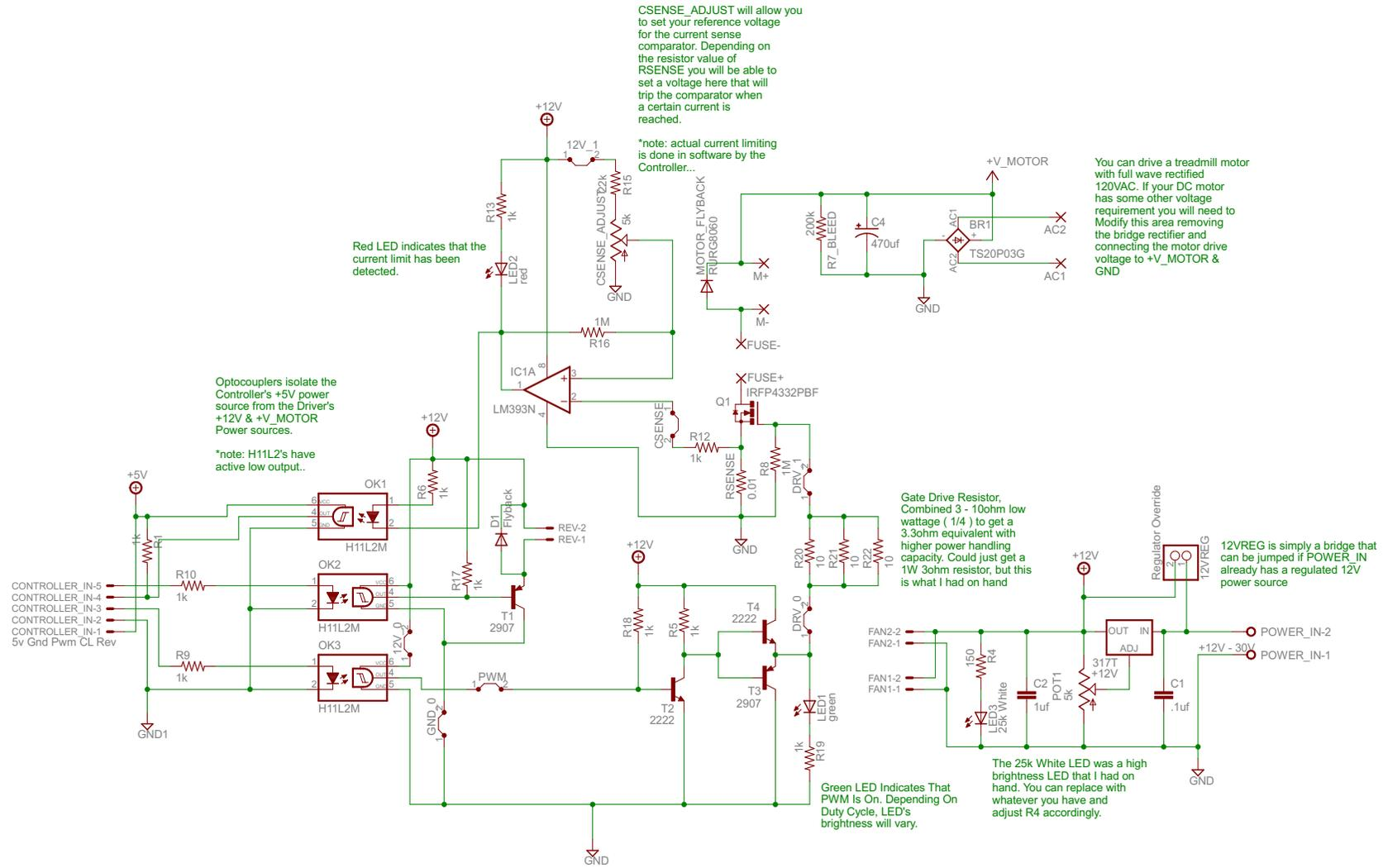
CSENSE\_ADJUST will allow you to set your reference voltage for the current sense comparator. Depending on the resistor value of RSENSE you will be able to set a voltage here that will trip the comparator when a certain current is reached.
