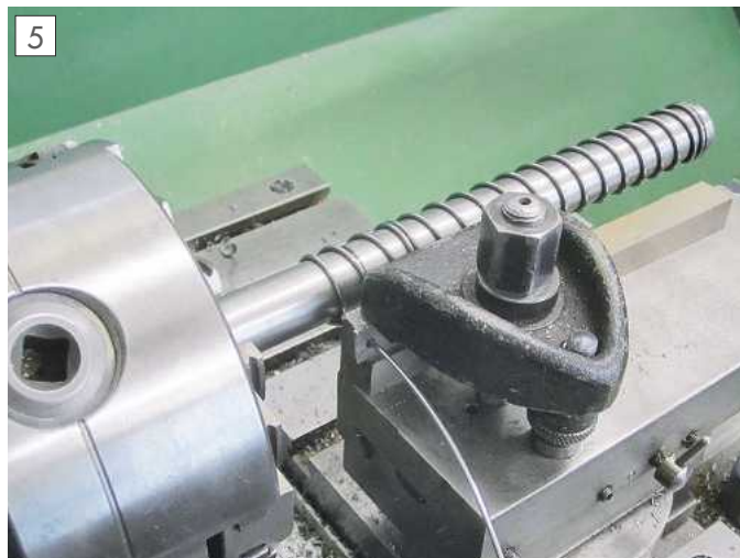
Spring winding on the lathe.
