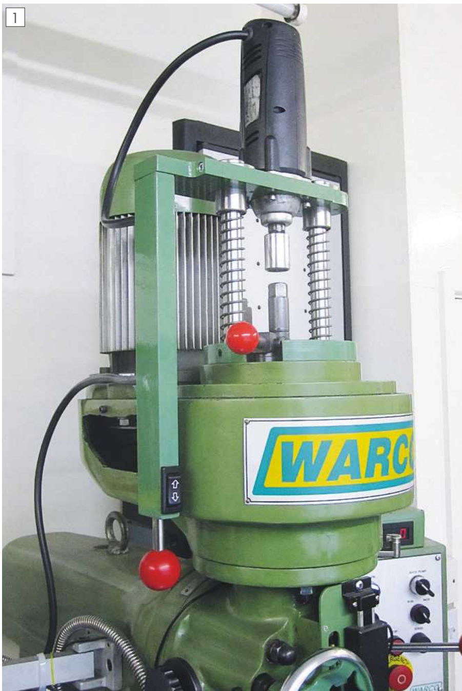
The completed power drawbar.
