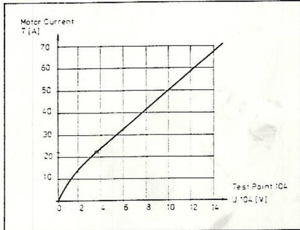
Fig. 13: Limiting Current of the Motor as a Function of the Voltage U 104
