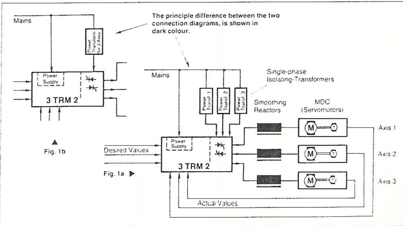
Fig. 1a: Connection Diagram for 3 Drive Axes with 3 Power Transformers
