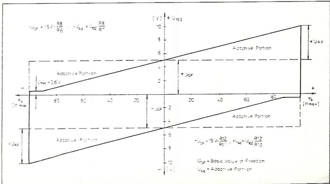
Fig. 3: Output-Voltage Range  $U_{103}$  of the Speed Controller as a Function of the Speed
