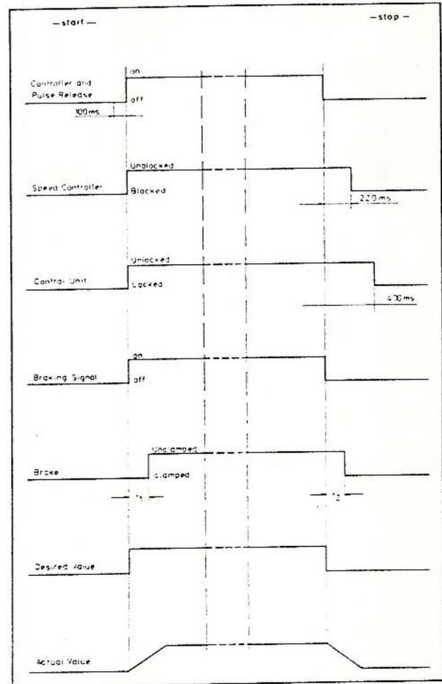
Fig. 14: Signal Sequence: Start-Stop-Operation
