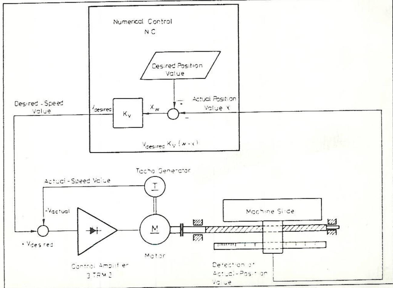
Fig. 15: Functional Diagram of the Position Control System
