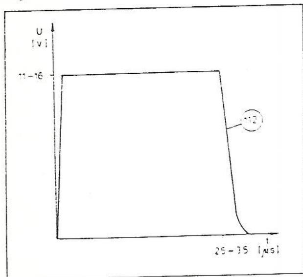
Fig. 6: Output Signals of a Trigger Pulse Generator
