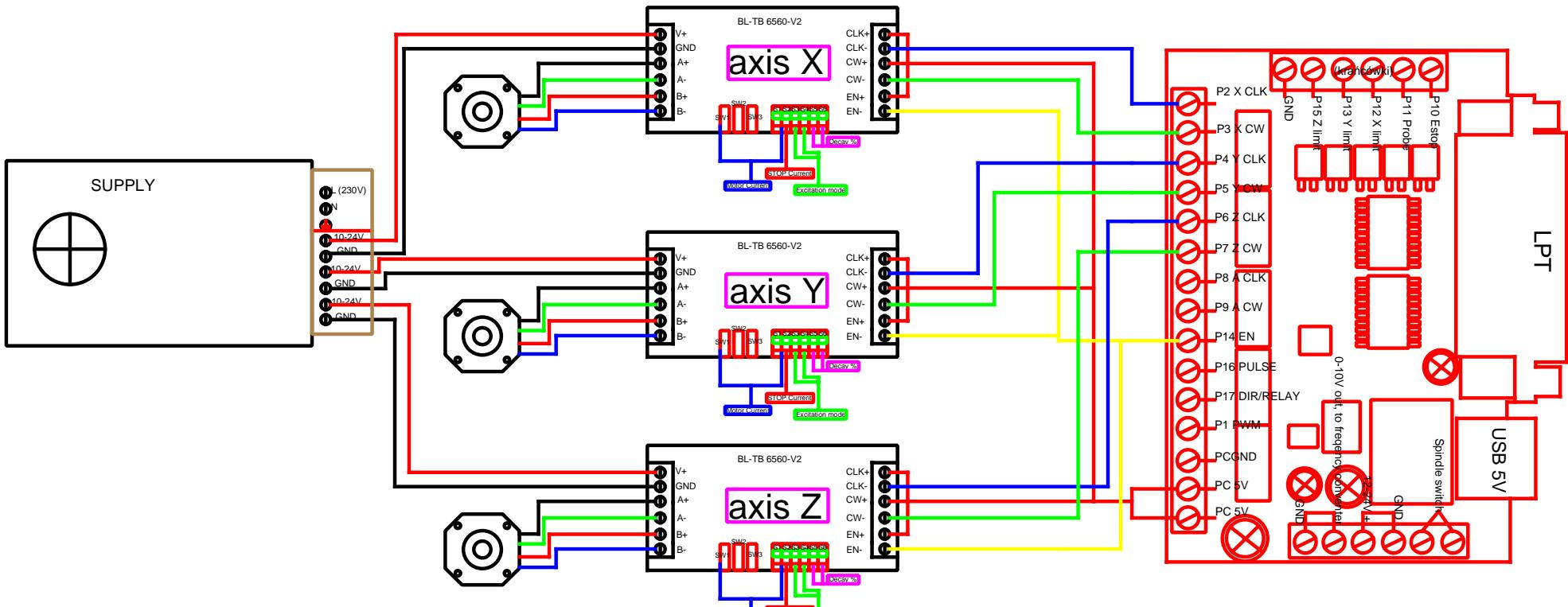
V1.1 when pcb driver is broken (P7-Z to P9-A, change mach pin)
