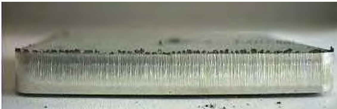
Gas pressure too high - .250 thick
