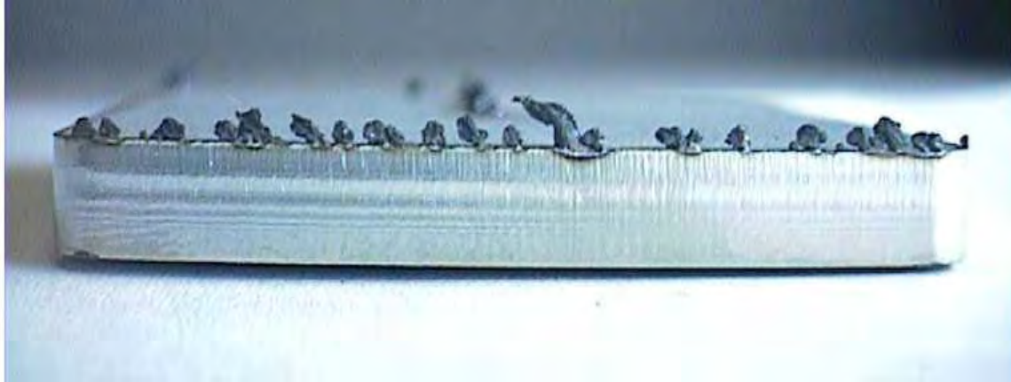
Cutting speed too slow - .250 thick
