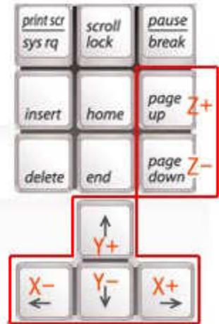
PS: you can use the keyboard to control the direction of the axis, and also you can use the manual control keyboard of Mach 3 by using the mouse to control the movement of the X, Y, Z axis.
