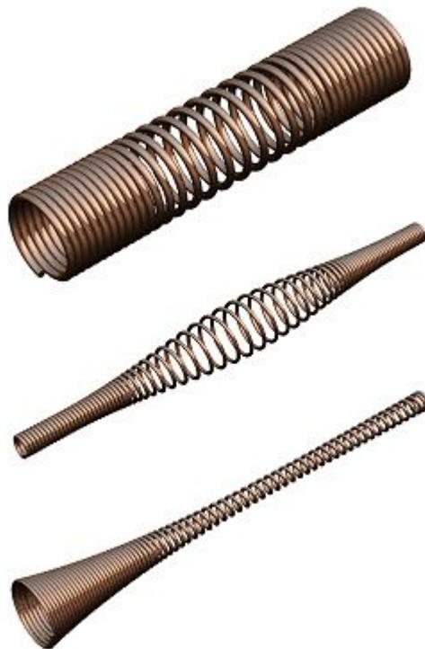
**Helical springs of variable radius and pitch using law functions**
