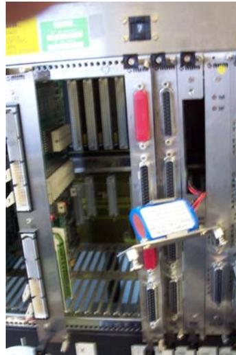
2. Remove battery and disconnect from connector (dispose of battery properly following State and Federal environmental guidelines).
