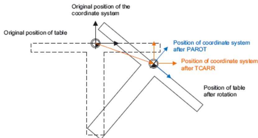
TOOLCARR.SPF(CUST\_800 is the name used in current CYCLE800.SPF) It moves and rotates the tool or table according to the input mode. Currently it is implemented for M20 M40 M41 cases.
