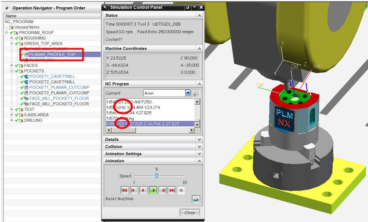
The example shown below (POCKET2\_PLANAR\_CUTCOMP, example sim05) is an alternative method when machining within a plane which is not aligned with xy, yz, or zx. Here, the working plane is not defined by a ROT statement; circular or cut comp output would not work and therefore are deactivated in the operation.
