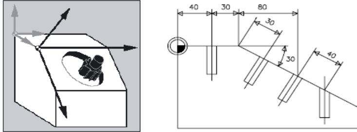
Working with swiveling cycles will make the life easier and let the controller do the work. In the following subchapters it is explained in detail how the swiveling Cycle PLANE Spatial on Heidenhain controllers and the CYCLE800 on Sinumerik S840D controllers work and how this is implemented in the CSE and the OOTB examples. In addition you will see a section how this is configured and can be reused for a different machine tool.
