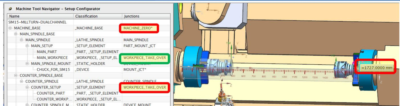
To achieve the mounting of the work piece from the main to the sub spindle the subprogram part\_takeover.spf located in the subprog folder of sim15 takes the responsibility. The kernel
