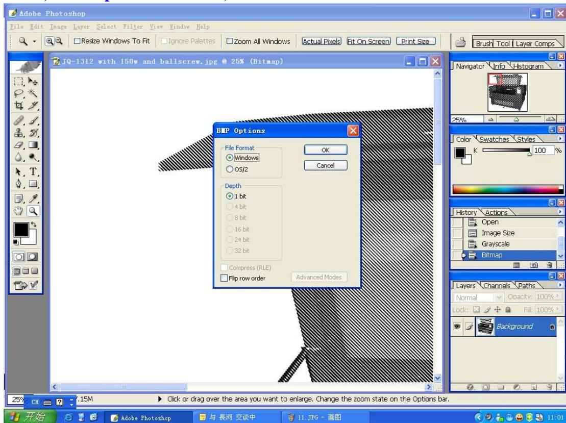
Tenth, open the Laser cut software, import the BMP picture. Then press this button
