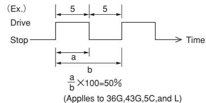
The gearhead is assembled with a fixed shaft about which a gear revolves and transmits power. It is not suited to continuous drive. You should maintain the duty ratio between ON and OFF states at no more than 50%, with the maximum ON state not exceeding 5 seconds.
