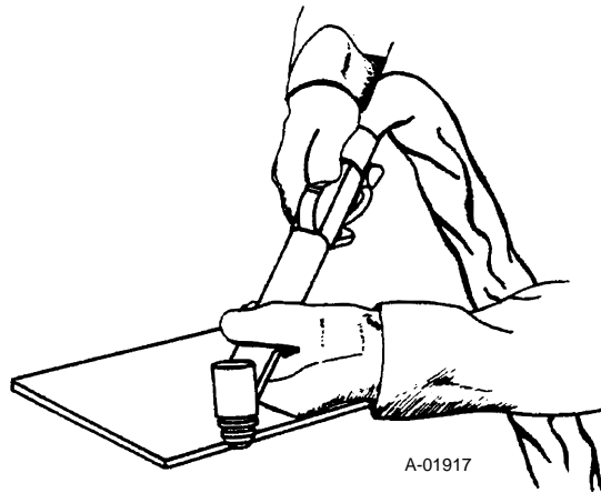
Figure 3-B Positioning the Hand Torch for a Cut
