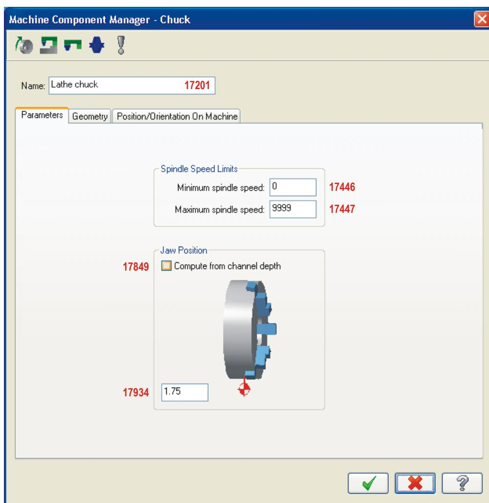
*Chuck geometry (parametric) dialog box*
