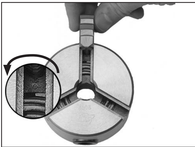
Figure 14. Lead thread.
