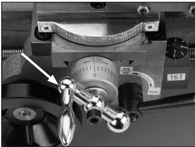
Figure 21. Cross slide handle and scale.
