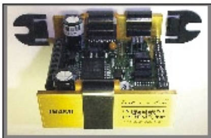
Figure C.2-A: Clips being installed on an IM805
